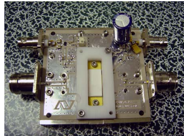
RF Test Board
